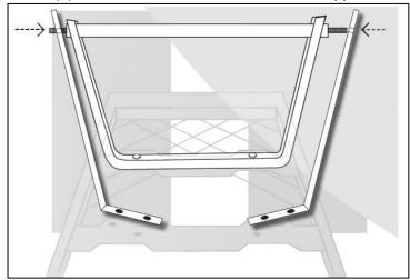
Attach using Rear Axle Braces using four Carriage Support Bolts, Washers & Nuts (18) x4.
