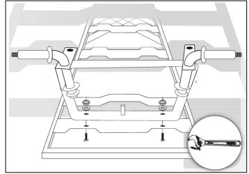
**STEP 4**Attach the Steering Link Connector (12) to the Front Axle Support arms, using 2x Bolts, Washers and Nuts (19). The connector should sit over the axle as pictured.
