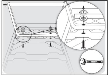
Place the Right (7) and Left (8) Rear Axle Braces onto the Rear Axle Support
