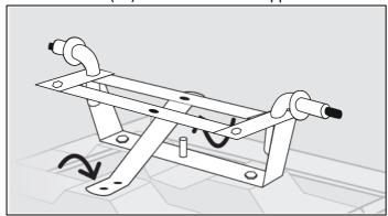
Fix the Central Front Axle Brace (10) to the Bed using 2x Carriage Bolt, Washer & Nut (18).
