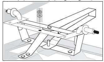
Slide the Large Washer (23) over the Front Axle Support (9) protruding leg and slide the Split Pin (16) through the hole. Split open the Pin legs to secure.
