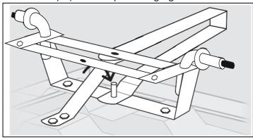
Position the straight arm of the Centre Front Axle Brace (10) between the Yoke (11) & Front Axle Support (9).
