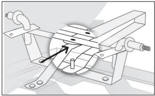
**STEP 7**Fix the Yoke (11) & Centre Front Axle Brace (10) to the Front Axle Support (9) using Bolt, Washer & Nut (19).
