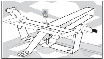
Fix the Steering Link Connector (12) to the Yoke (11) using Carriage Bolt, Washer & Nut (18).
