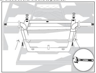
**STEP 5**Position the Central Front Axle Brace (10) to the Front Axle Support
